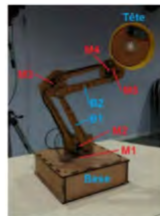
Figure 2 : Composition de la lampe [3]
